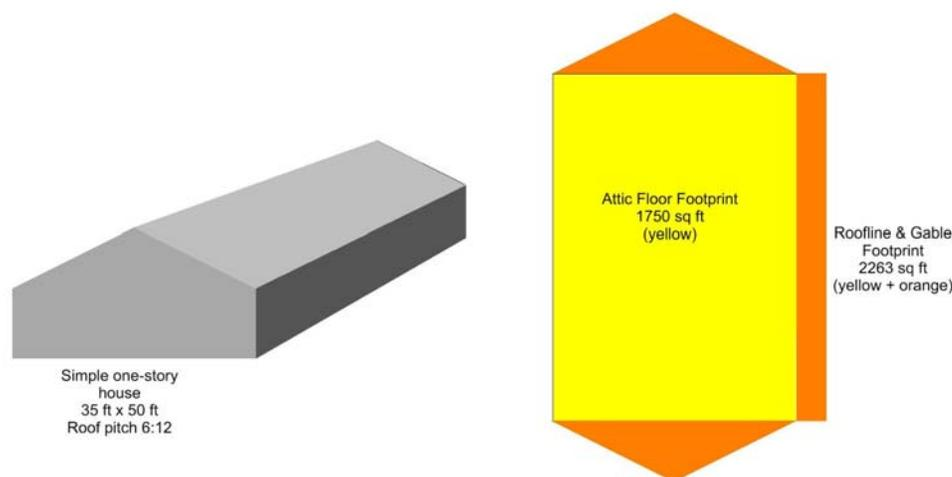
**Figure 2:** Comparative insulated areas for vented and unvented attic
